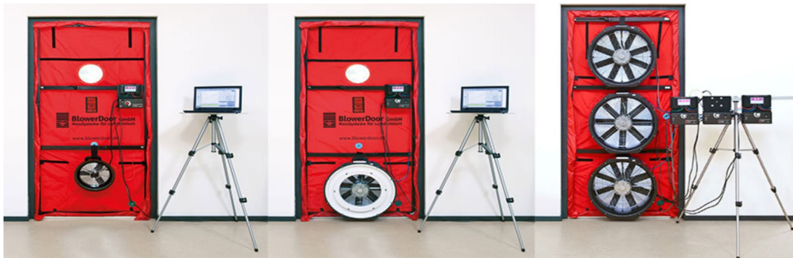
Figure 7 Types of Blower Door test equipment according to the power required.
