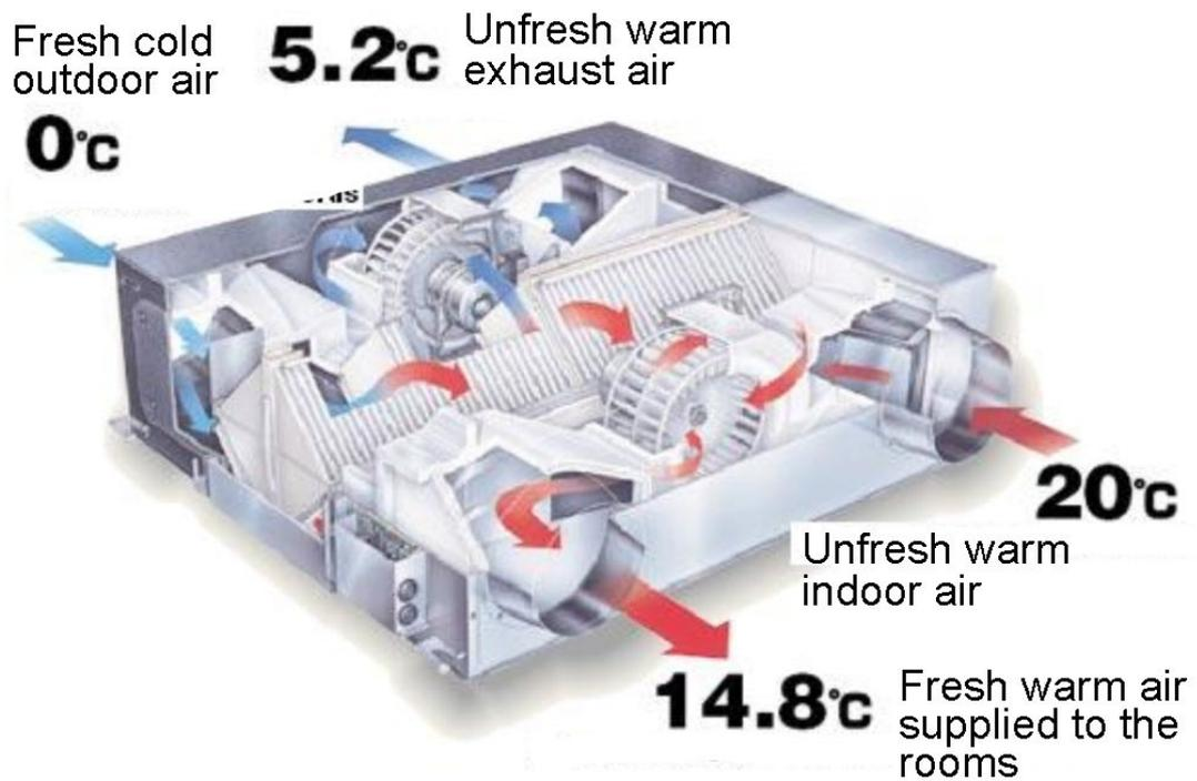
Figure 11 Operating principle of the recuperator.
