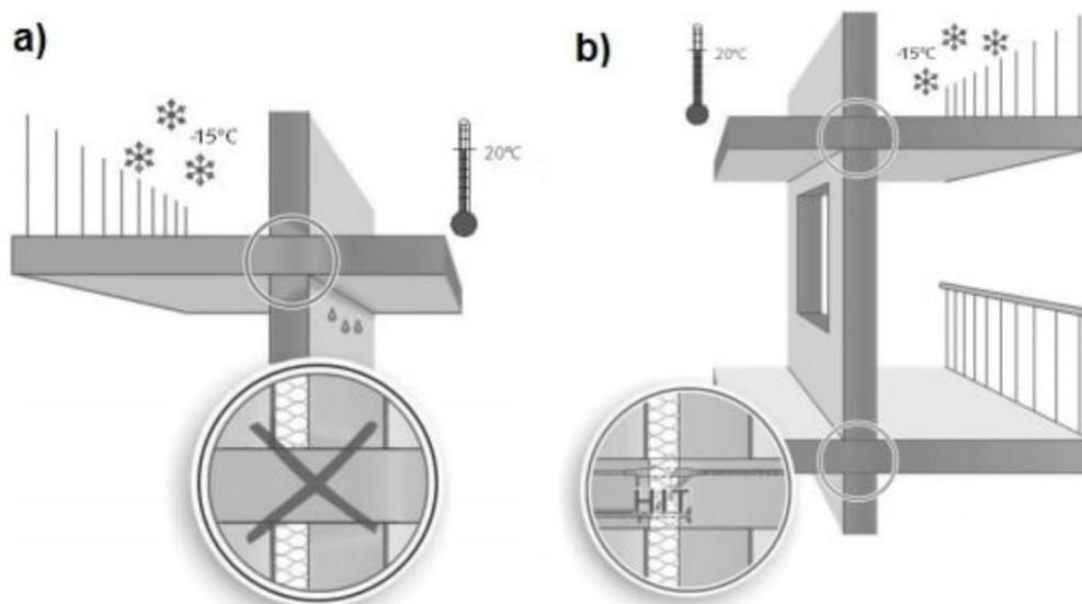
Figure 18 Balcony panel installation solution without thermal bridge.
