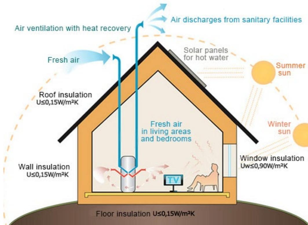
Figure 1. The five key principles of Passive House.
