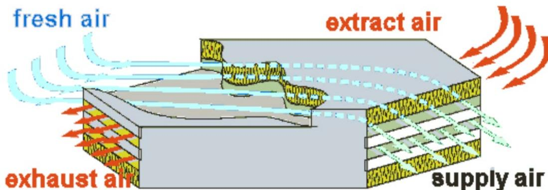
Figure 12 Principle diagram of a plate heat exchanger.
