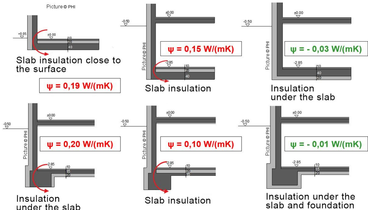
**Construction without thermal bridges:  $\psi \leq 0,01 \text{ W/(mK)}$**
