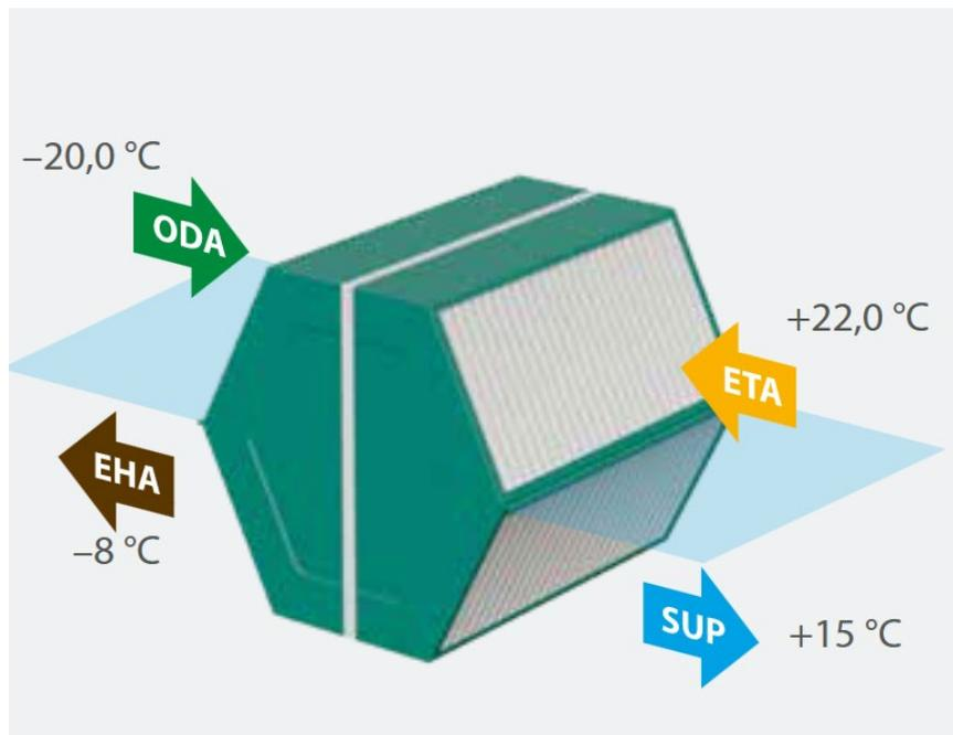
Figure 13 Principle diagram of a cross-flow heat exchanger.
