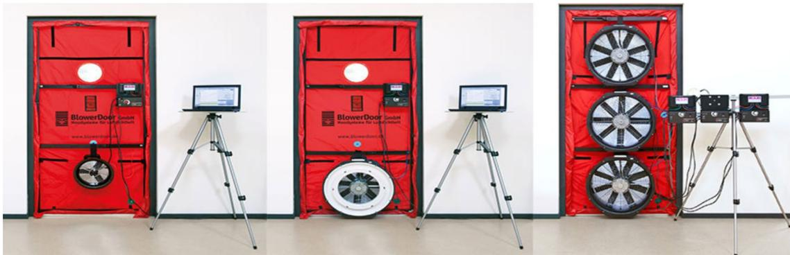
Figure 7 Types of Blower Door test equipment according to the power required.
