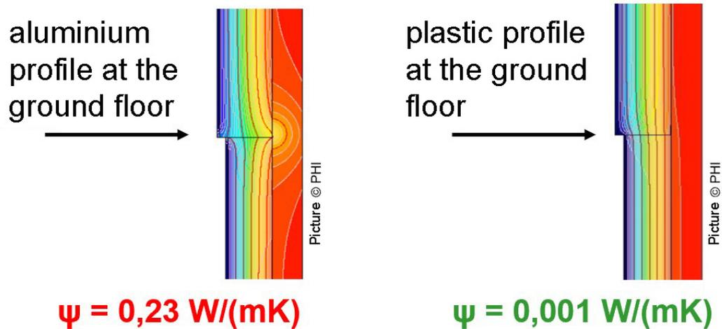
Figure 17 Thermal bridging with different materials.
